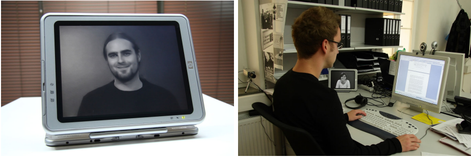
Fig. 1. The perFrame prototype was implemented with an HP Compaq tc1100. The keyboard is rotated to the backside and serves as a stand for the picture frame. For our study the perFrame prototype was deployed on the employees’ desks. The camera for the Wizard of Oz observation can be seen on the left edge of the right picture.
